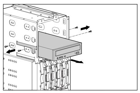
Figure 2-22. Removing a drive from the removable media area
